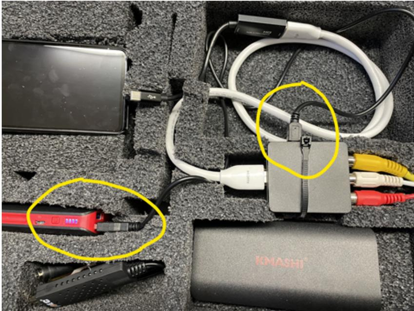
Make sure the HDMI cable is plugged into the adapter and to USB-C port on the phone:
